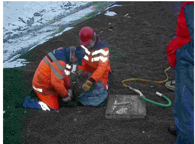
Figure 8 Sampling of compacted material
