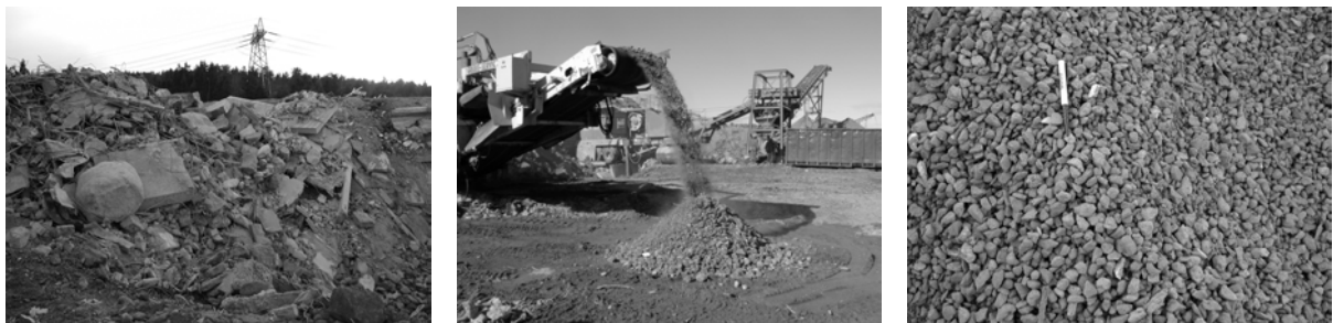
Figure 1 After crushing and sieving the crushed concrete becomes useful recycled aggregates for concrete (Picture: Bente Lillestøl, Veidekke ASA)
