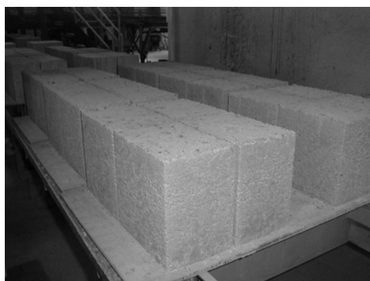
Figure 5 Building blocks with 30 % recycled aggregates (0-4 mm) (Picture: Bente Lillestøl, Veidekke ASA)
